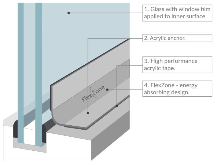
The Flexi25 Glass Anchoring System is installed on all four sides of the window test specimens with adhesion to the powder coated aluminium frame and adhesion to the inner surface of the film.
